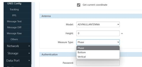
The "ah" (antenna height, which is actually the bottom height) in the RTCM1006 message output is the result calculated through the antenna information parameters filled in the [Positioning Configuration] page. Its value range is 0.0000-6.5535. If the converted value is not within this range, the page will prompt "Invalid parameter" during application. The conversion methods for the three antenna height measurement modes are as follows:
