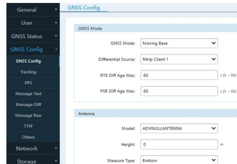
Antenna model and height information can be determined based on the specification manual or by consulting technical personnel. The current antenna configuration model is generally default; "Measurement Method" is available for selection, but "Phase" is generally default. Display as follows:
