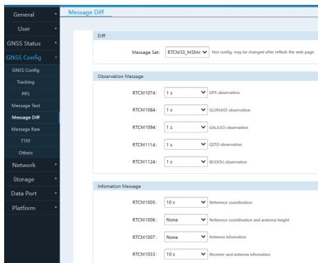
(3) Set raw data output at 1 Hz (1 second per output). The display is as follows:
