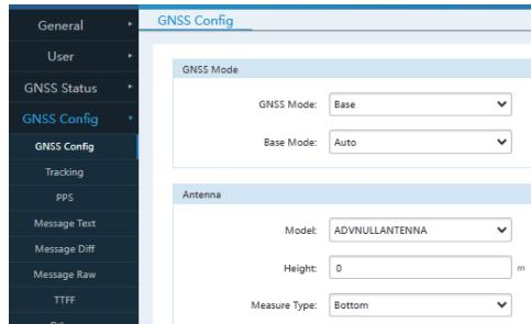
In Repeat Coordinate mode, you can manually input the antenna's location coordinates to start the base station, or check "Get Current Coordinate" to obtain the NET660i's current single-point coordinates for base station startup. Display as follows:
