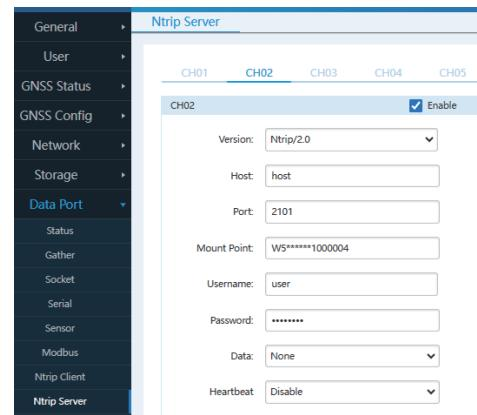
(4) Set Ntrip Server connection 2 to use the Ntrip/2.0 protocol to send RTCM33 to a CORS server. Select positioning differential data as the data source, as shown below:
