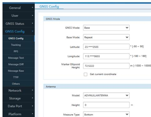
You can also select the base station (motion direction finding) mode, as shown below.
