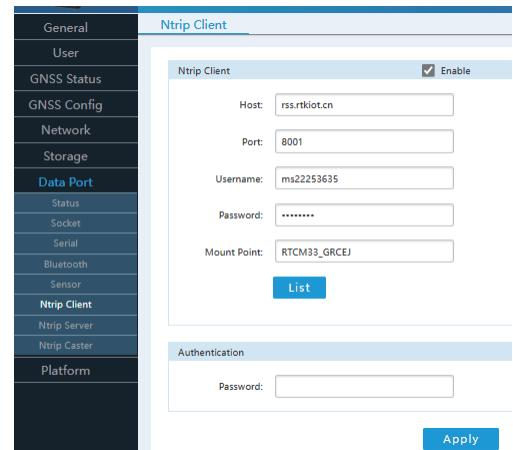
(5) Obtain the access point, select the mount point to be accessed, and click "List" to retrieve the differential data of this access point from the server. The display is as follows:
