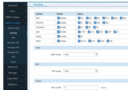
SBAS (Satellite-Based Augmentation System) improves the accuracy and reliability of satellite navigation systems. It defaults to automatic mode, automatically using the optimal satellite-based augmentation system based on actual conditions, or manually select a single SBAS.
